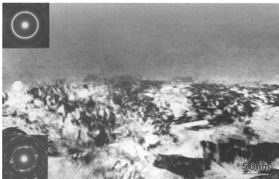
Figure 7 Interface region of Tribaloy T-800 sprayed by HVOF process on nickel-base superalloy substrate.
