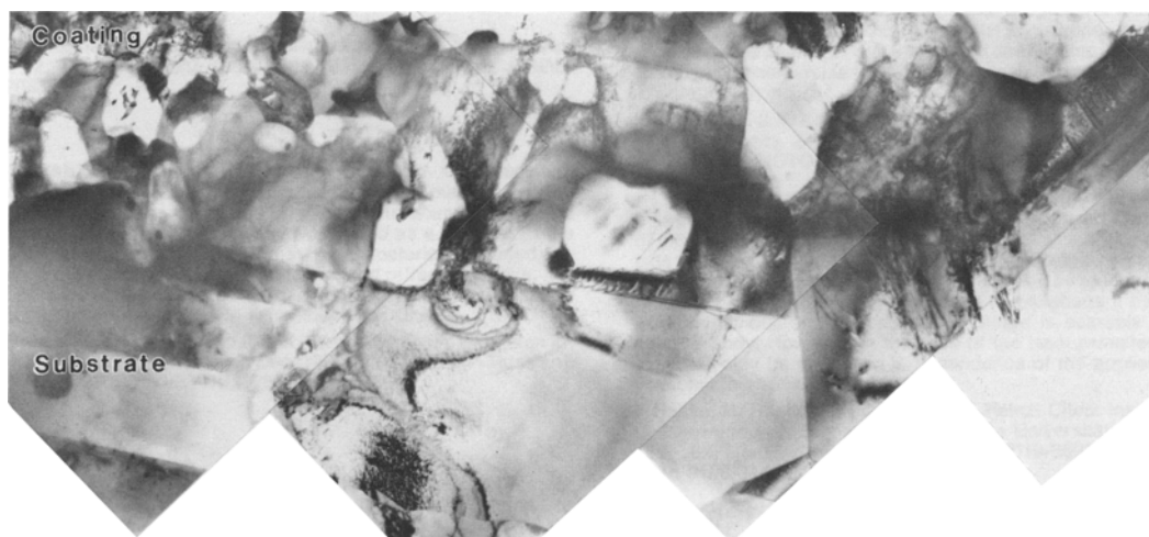
Figure 9 Microstructure of T-800 coating on nickel-base super-alloy after heat treatment.
